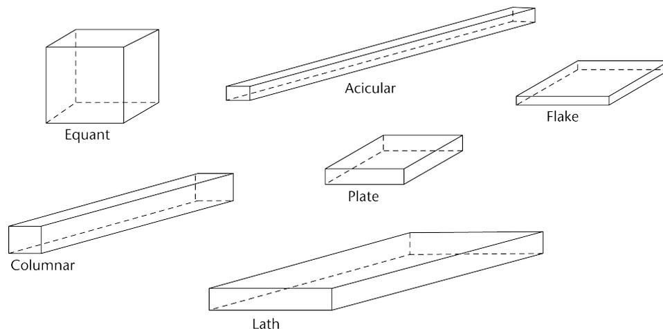
Figure 2. Commonly used descriptions of particle shape.
